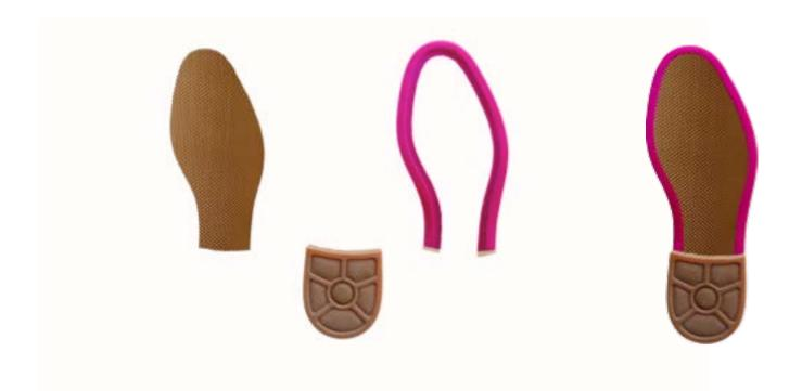
how we can mould a sole in pieces and assemble it on a modified last and insole
