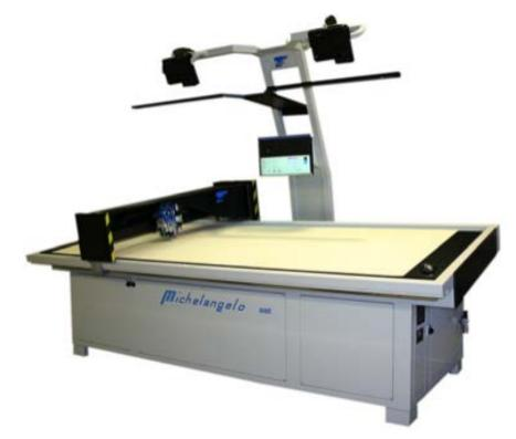
Insoles and soles can now be cut by a CAD/CAM system with the information controlled by the m2m software
